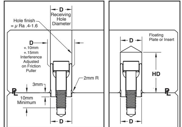
Recommended interference fit is .1 to .15mm larger than the receiving hole. To adjust the Friction Puller, rotate the screw clockwise and measure bulge to achieve the proper fit. Further adjustments can be performed with 1/4 turn increments, lining up the reference arrows on the fastener to the resin.
