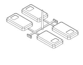
With ECOVENT application a big gas venting area is set up at the end of the runner that allows the gases produced during the melting process to flow through the system instead of flowing into the cavity.
